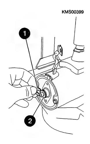
Checking and adjusting armature axial clearance
